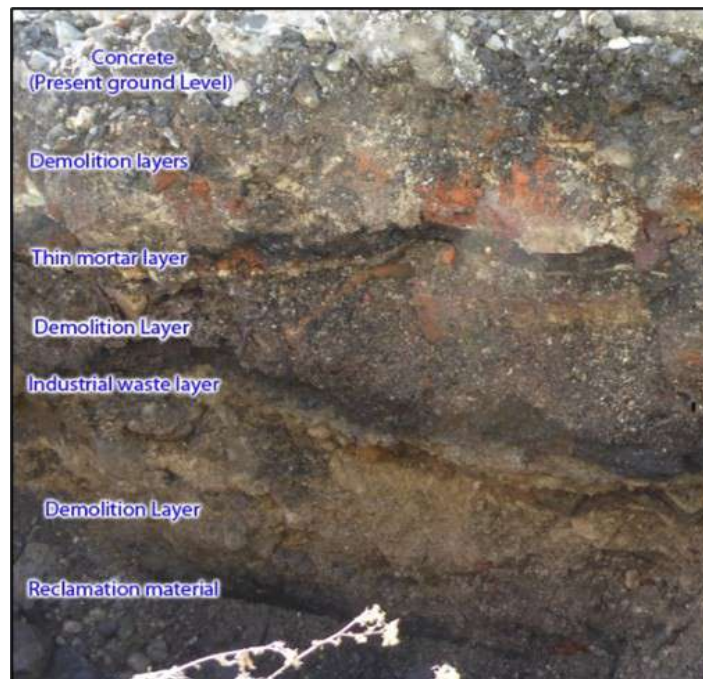
Plate 1 Typical cross section of upper levels, photo of TP5 of the first 1.5m of the pit
