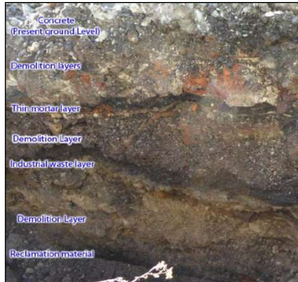
Plate 9 Typical cross-section of upper levels, photo of TP5
