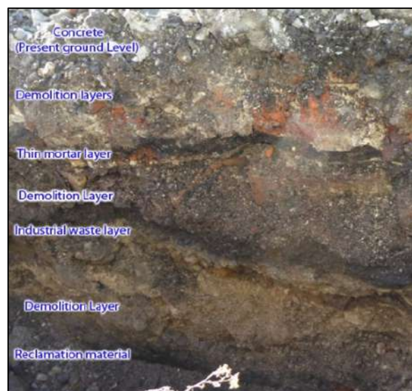
Plate 7 Typical cross section of upper levels, photo of TP5
