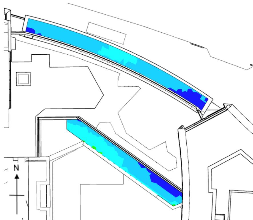
Fig. 4.2.3 – Lawson Criteria Results for Block B2 L08 balconies as initially designed.
