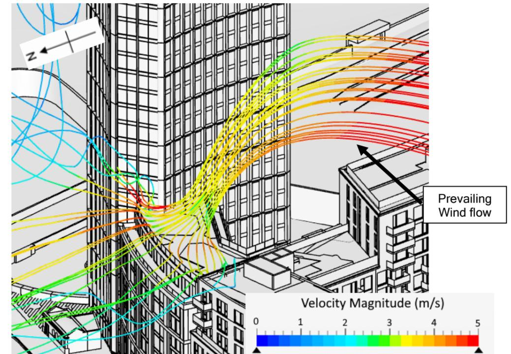
Fig. 3.1.1 – Wind velocity streamlines from prevailing SW wind direction across the roof the Block B2 for the initial design.
