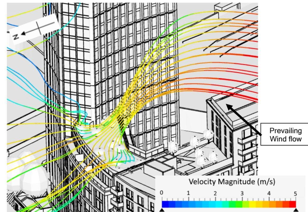
Fig. 3.1.2 – Wind velocity streamlines from prevailing SW wind direction across the roof the Block B2 for the finalised design.
